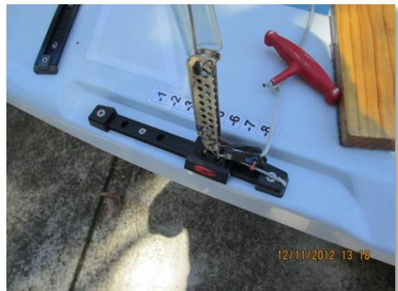
The standard setting, which gives you range from 0-18/20 knots (exact range depending on crew weight) is measured with the rig pulled fully back.
